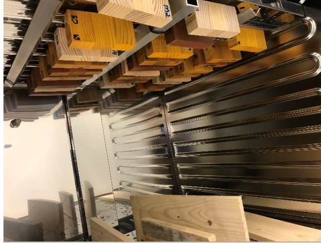
Figure 3.8 Placement of test samples on the top of chamber.
