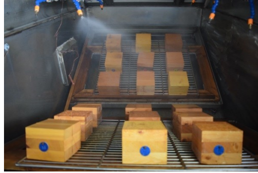
Figure 3.3 Weathering apparatus containing blocks fixed at 45° angles to holding racks.
